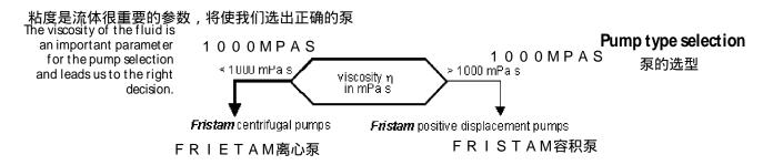
FRIETAM离心泵是装备开放式叶轮的,适合输送粘度小于1000的流体 *Fristam* centrifugal pumps are equipped with open impellers which are suitable for the transfer of liquids with viscosities up to 1000 mPas.
