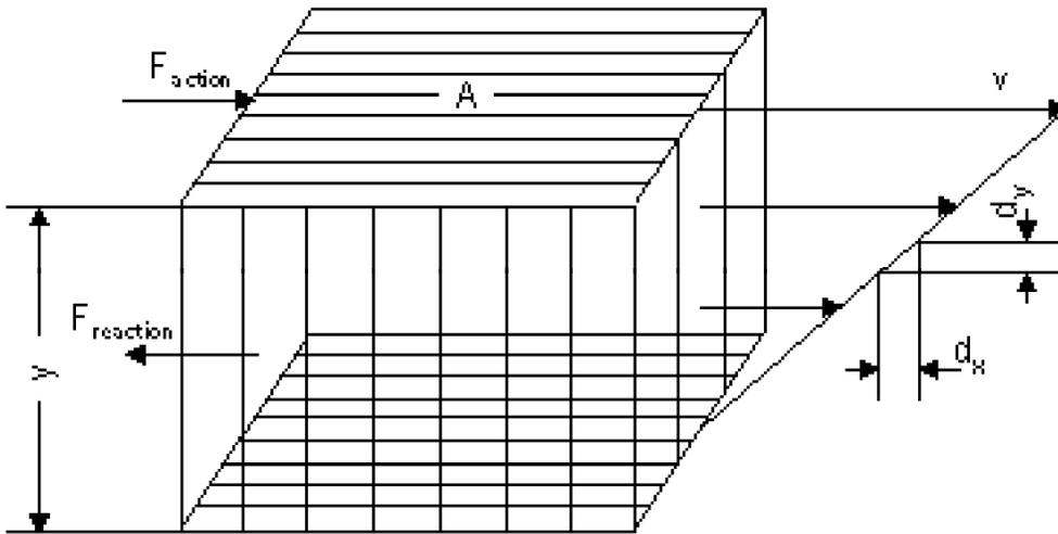
The ratio of F to A is called shear stress  $\tau$ . F 与 A 的比率叫剪切压力
