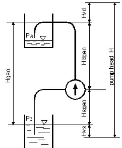
In order to ensure a correct operation of the pump the following condition must be given:
