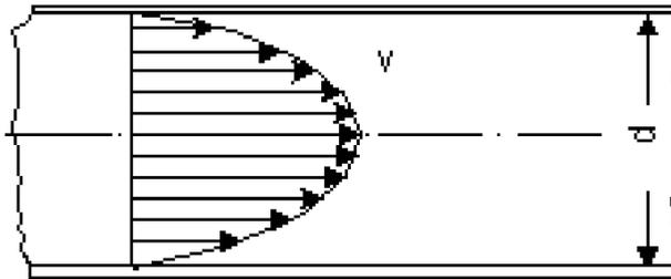
The roughness of the inside wall of pipes has no effect on the friction loss.
